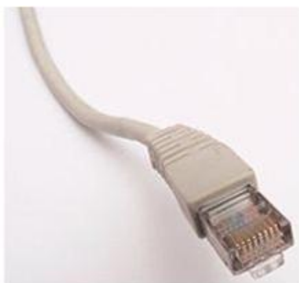
Figure 5: An 8P8C modular connector (often called RJ45) commonly used on Cat 5 cables in Ethernet networks
